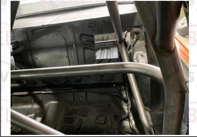
PHOTO 12 SHOULDER HARNESS ATTACHMENT - DRIVER
