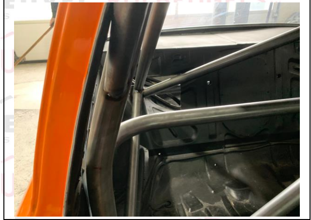
PHOTO 13 SHOULDER HARNESS ATTACHMENT - CO DRIVER
